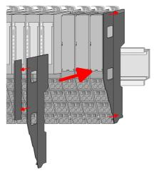
After mounting the whole system, to protect the backplane bus connectors at the last module you have to mount the bus cover, now. If the last module is a clamp module, for adaptation the upper part of the bus cover is to be removed.
