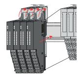
**6.** To mount the module group put it to the gap between the both modules and push it, guided by the stripes at both sides, to the mounting rail.
